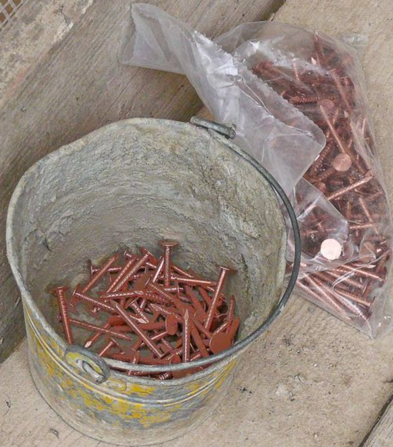
Copper nails for hanging the tiles
