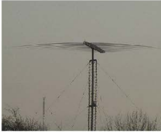
The Log Periodic Antenna is broadband and a very good back to front ratio
