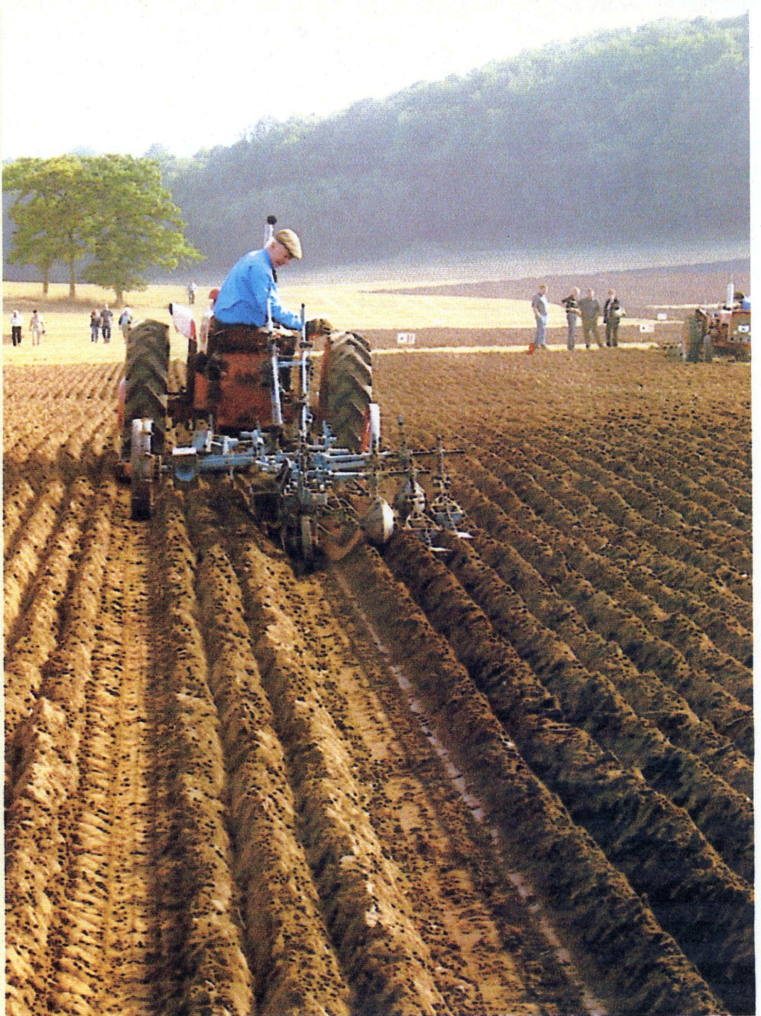
Above: International B250 or B275 tractors are ideal for 'high-cut' work, for the driver can just sit back over the diff and control the tractor with one hand, and the trailed plough with the other. This is another fine view of Douglas at work.
